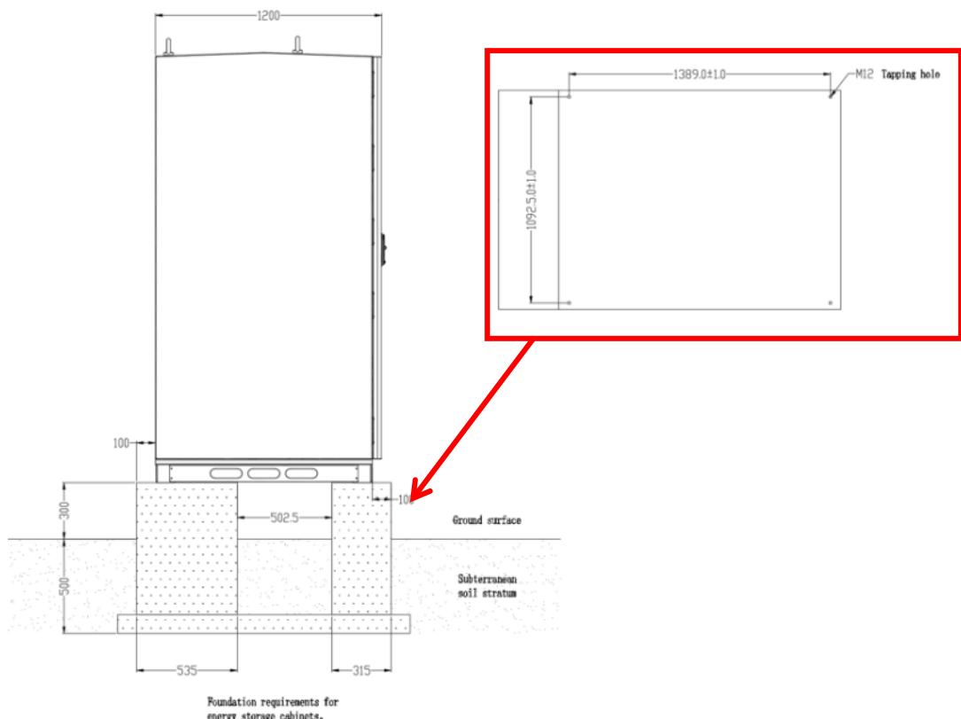
Figure 5-3 Base Fixing Diagram
