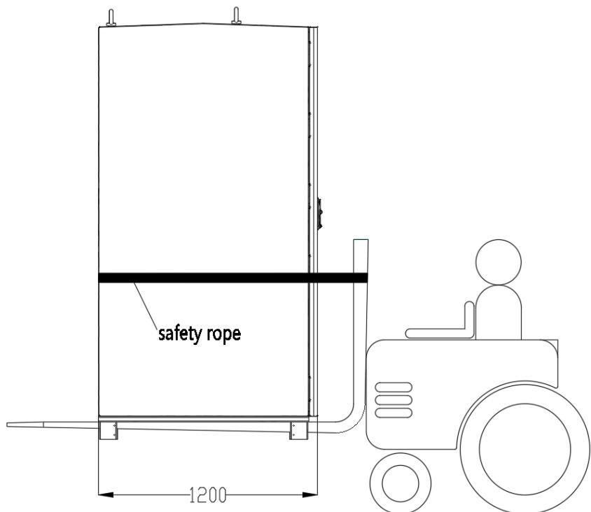
Figure 4-2 Forklift Installation Diagram for the Front/Back of the Energy Storage Cabinet
