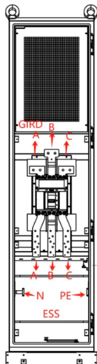
Figure 5-7 Wiring Diagram Inside the Combiner Box
