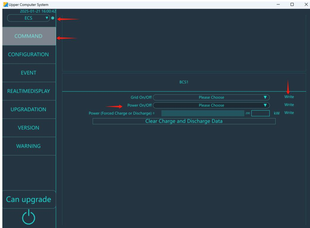
**Step 3** In the ECS display interface, check that the charging and discharging status of the corresponding device is stopped, confirming that the shutdown has been successfully executed.
