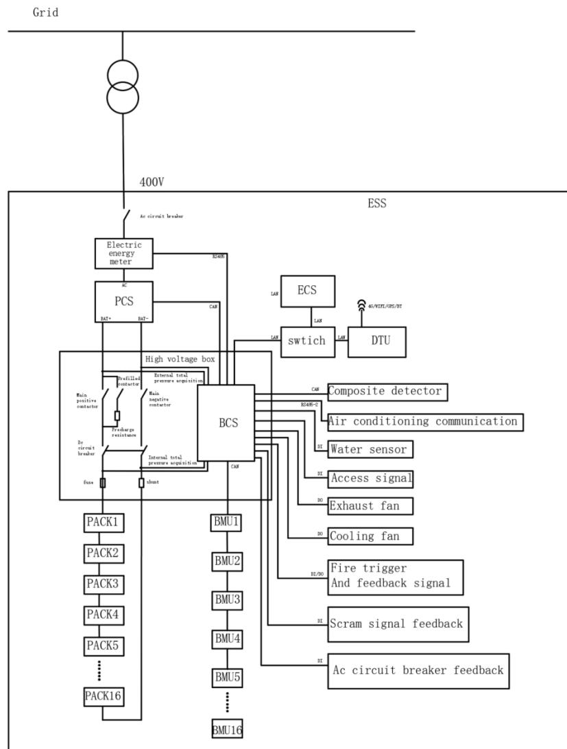
Figure 2-4 Energy Storage System Topology Diagram
