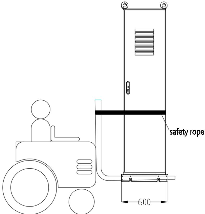
Figure 4-3 Forklift Installation Diagram for the Side of the Combiner Box
