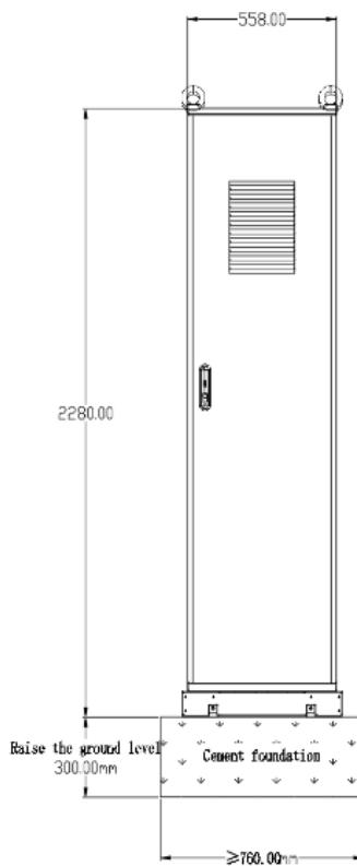
Figure 5-2 Combiner box fixing diagram
