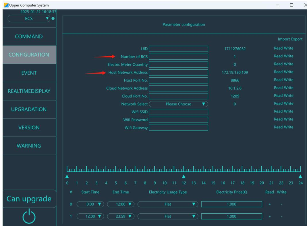
➤ In the BCS configuration interface, input the communication address of the BCS to complete the parameter configuration for communication between the upper computer and BCS.
